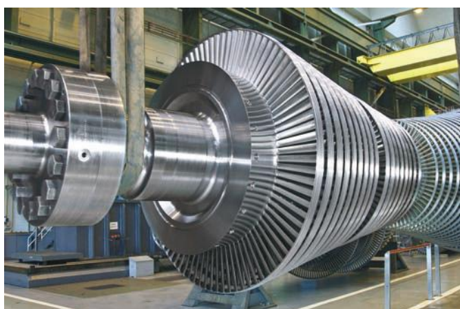
Figure 15.6 The rotor of a steam turbine
