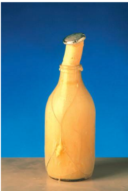
Figure 19.6 Result of the expansion of water on freezing
