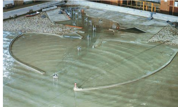
Figure 25.9 Model of a harbour used to study wave behaviour
