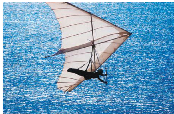
Figure 23.8 Once airborne, a hang-glider pilot can stay aloft for several hours by flying from one thermal to another.
