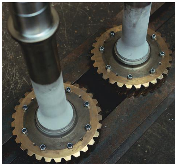
Figure 19.1 'Shrink-fitting' of axles into gear wheels
